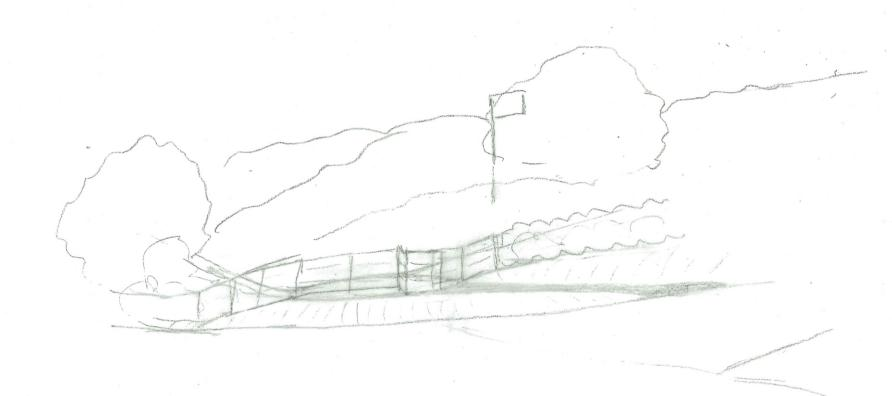
STEPS TO ENTRANCE REMOVED. BANK EXCAVATED SO THAT LINE OF LOWER PATH IS CONTINOUS WITH THE ENTRANCE. CLARITY OF DIRECTION.
