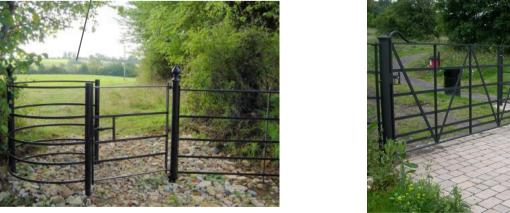
KISSING GATE ALLOWS PEDESTRIAN & PRAM ACCESS BUT PREVENTS MOTORCYCLE ACCESS.
